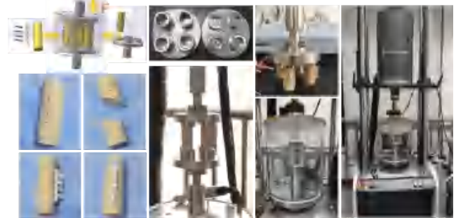
Fig. 1. Schematic diagram of cyclic mechanical loading degradation model of bone nail and bone plate.
