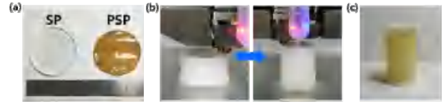
Fig. 2. (a) Comparison of macroscopic morphology of SP and PSP coated hydrogel; (b) 3D printed polymer stent; (c) PSP hydrogel-coated intestinal stent
