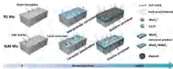
Fig. 1 Corrosion mechanism of SLMed Mo compared to bulk Mo.
