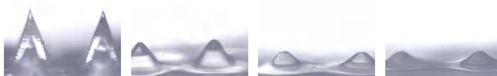
Figure 2 Schematic illustration of GelMA hydrogel microneedle degradation in vitro at 0 h, 24h, 48h, 72h.
